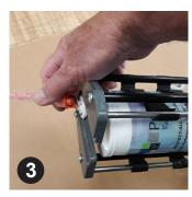
Install the mixing nozzle and secure with the previously removed cap.
