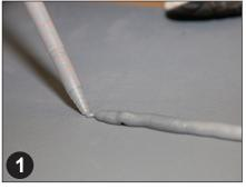
Dispense the Protect-All Rapid Weld onto scrap cardboard until a consistent color is achieved. Once this step has begun, you must continue to move product through the nozzle.
