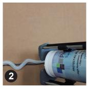
Using a piece of cardboard or scrap Protect-All, dispense the Protect-All Rapid Weld until Part A (white) and Part B (color) flow from the end.
